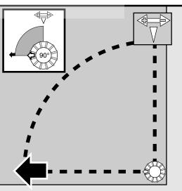
Align the right stop arrow to the right side of the watering arc.
