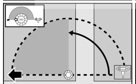
The watering area is between the cap arrow and the right stop arrow on the arc adjustment ring. This example is set to 180°.
