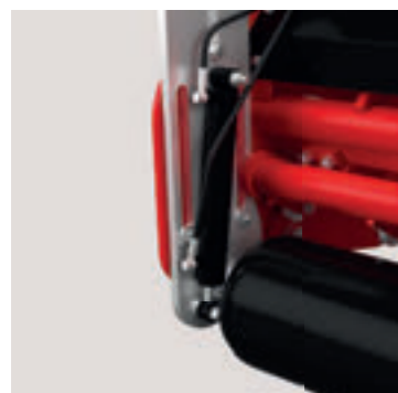
Hydraulic depth control
