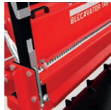
Levelling bar to created a smooth and level finish.
