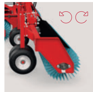
Brushes can be rotated in either direction.
