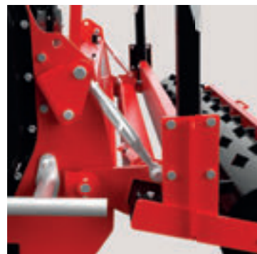
Moveable rear packer roller.
