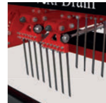
Tine head with multiple tine options.
