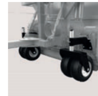
Optional caster wheels for hard surfaces.
