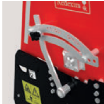
Adjustable seed gate to cater for multiple seed types.
