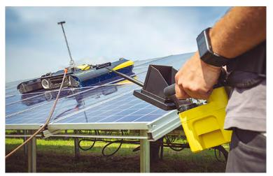
No work at height: remote control from ground level
