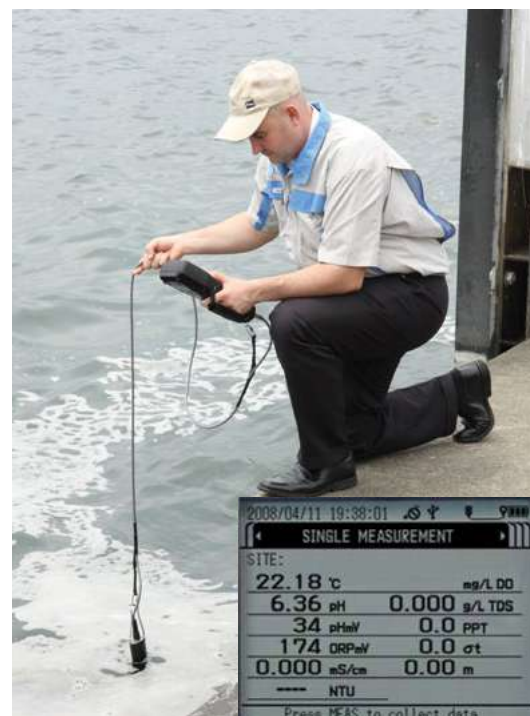
Water quality monitor displays 11 parameters simultaneously
