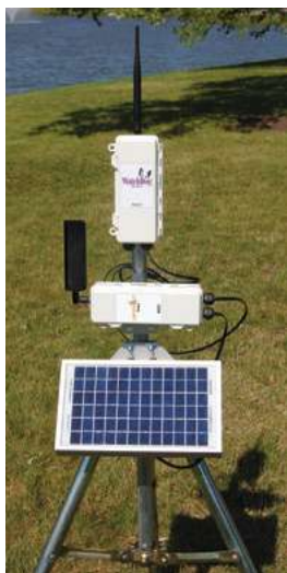
3928M DataScout Cellular Modem Mounted with a WatchDog Retriever
